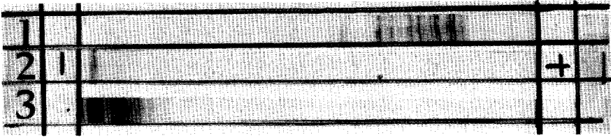
Fig. 6. Flat bed isoelectric focusing in 1% agarose gel ( 0.5 \text{ mm} \times 10 \times 24 \text{ cm} ) (pH 3-10). Focusing was performed at 15 W for 1 h. The gel was fixed in a solution of trichloroacetic acid and sulphosalicylic acid and stained with Coomassie Brilliant Blue. (1) Raw timothy pollen extract; (2) Fr. C from the Mono S column (Fig. 2); (3) Fr. I from the CM-Sepharose CL-6B column (Fig. 4).
